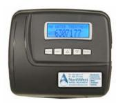
Clack Dot Matrix control valves include a microprocessor and backlit screen with push button settings for ease of use. The metered control valve provides greater efficiency and reduced salt usage, because regeneration of the water softener is based on water consumption. The Matrix control valve indicates a "call for service" alarm when a scheduled maintenance is recommended.
